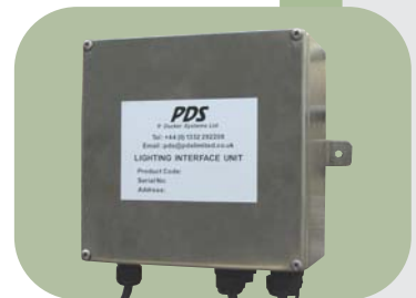
LIUs INTERFACE BETWEEN EACH DALIBUS (MAX. 64 LUMINAIRE BALLASTS) AND THE MAIN COMMUNICATIONS NETWORK
